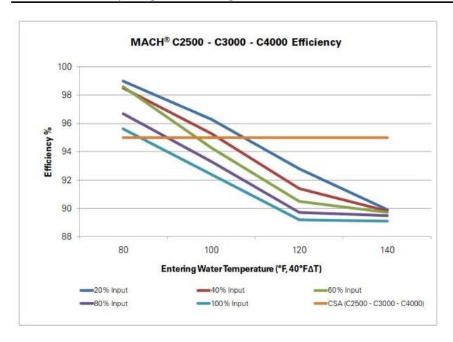
Figure 4.2.1 - Mach C4000 Boiler Part Load vs Entering Water Temperature Efficiency
